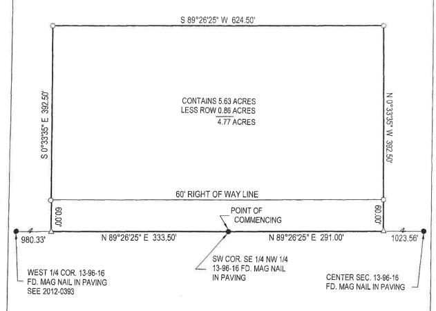
CONTAINS 2.62 AC INCLUDING 0.40 AC. IN ROW IN SE 1/4 OF NW 1/4 AND 3.01 AC. INCLUDING 0.46 AC. IN ROW IN SW 1/4 OF NW 1/4 IN SECTION 13
